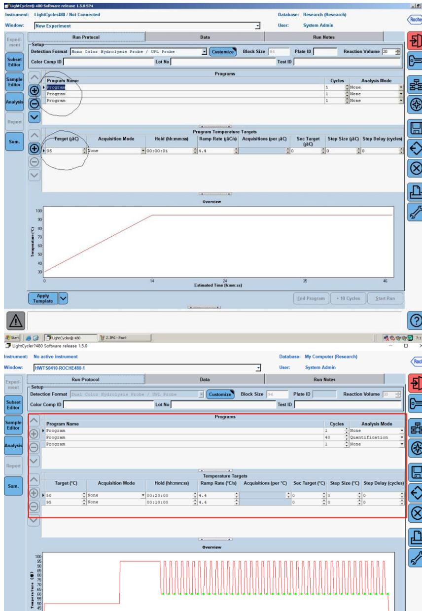
(5) Save the program as a template by clicking **Save As Template**. The template can be used for future experiments by clicking **Apply Template** (see screenshot below).
